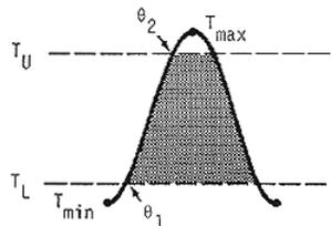
$$\begin{aligned} \text{°D} &= \frac{1}{\pi} \left\{ \left( \frac{T_{\max} + T_{\min}}{2} - T_L \right) (\theta_2 - \theta_1) + \alpha [\cos(\theta_1) - \cos(\theta_2)] + (T_U - T_L) \left( \frac{\pi}{2} - \theta_2 \right) \right\} \\ \theta_1 &= \sin^{-1} \left[ \left( T_L - \frac{T_{\max} + T_{\min}}{2} \right) \div \alpha \right] \\ \theta_2 &= \sin^{-1} \left[ \left( T_U - \frac{T_{\max} + T_{\min}}{2} \right) \div \alpha \right] \end{aligned}$$
