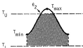
$$\text{°D} = \frac{1}{\pi} \left\{ \left( \frac{T_{\max} + T_{\min}}{2} - T_L \right) \left( \theta_2 + \frac{\pi}{2} \right) + (T_U - T_L) \left( \frac{\pi}{2} - \theta_2 \right) - \left[ \alpha \cos(\theta_2) \right] \right\}$$
